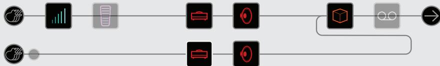
This new Input block can be assigned to a completely different input. This routing can be used for mixing a guitar and vocal or the models and magnetic pickups in a connected Variax guitar, each with their own processing blocks.
