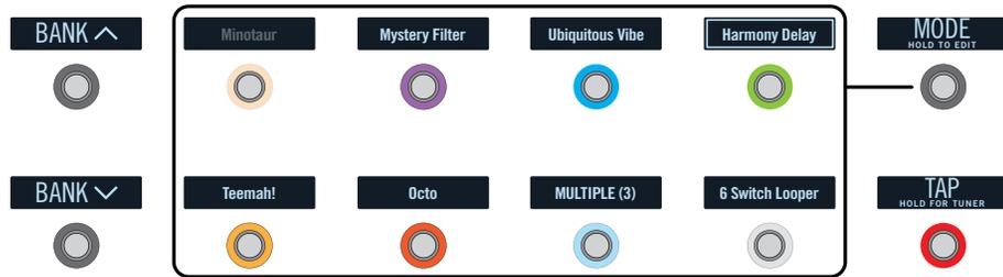
**NOTE:** If a switch is assigned to multiple blocks or items, its scribble strip reads “MULTIPLE (X),” where X is the number of assignments, and stepping on the switch turns them all on and off. If some blocks are on and some are bypassed, stepping on the switch toggles each block’s bypass state.
