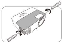
13. Tighten the screw that secures the lamp cover.
