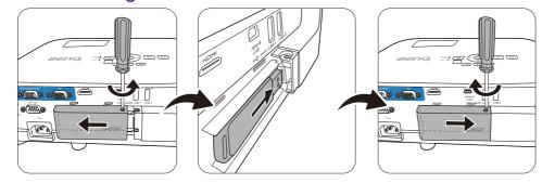
The projector only supports Wi-Fi and/or Bluetooth connections when the wireless dongle (WDR02U) is installed.
