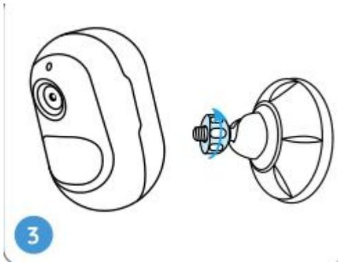
**Step 4.** Adjust the camera's angle to get the best field of view.
