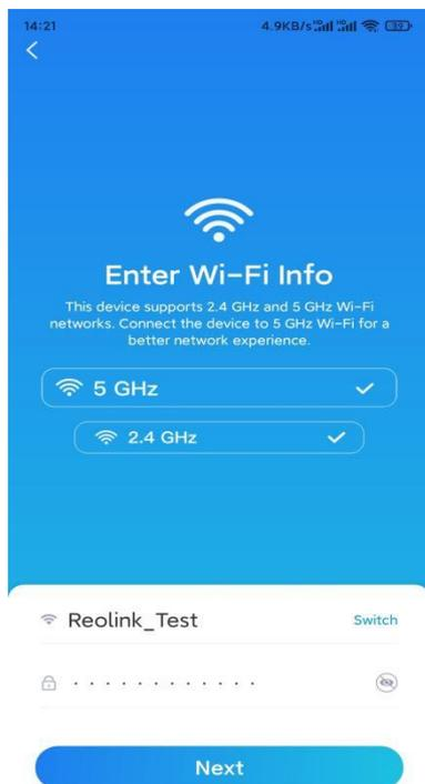
**Note:** Only Argus 3 Pro, Argus PT (5/2.4GHz), Reolink Duo (Battery) and Reolink TrackMix support 5GHz/2.4GHz Dual-Band WiFi connection.
