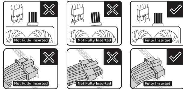
Please make sure the 12V-2X6 Cable has been fully inserted into the cable on the power supply unit and graphics card before use. Leave sufficient space for connecting the 12V-2X6 cable, do not bend or squeeze the cable.
