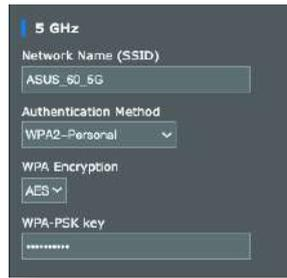
The screenshot shows the configuration interface for a 5 GHz wireless network. It includes a 'Network Name (SSID)' field with the value 'ASUS\_60\_5G', an 'Authentication Method' dropdown menu set to 'WPA2-Personal', a 'WPA Encryption' dropdown menu set to 'AES', and a 'WPA-PSK key' field with a masked password '\*\*\*\*\*'.
