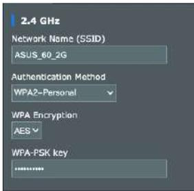
The screenshot shows the configuration interface for a 2.4 GHz wireless network. It includes a 'Network Name (SSID)' field with the value 'ASUS\_60\_2G', an 'Authentication Method' dropdown menu set to 'WPA2-Personal', a 'WPA Encryption' dropdown menu set to 'AES', and a 'WPA-PSK key' field with a masked password '\*\*\*\*\*'.
