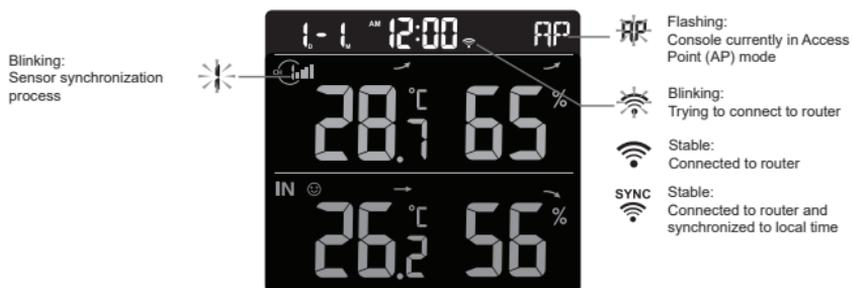
4. The wireless sensor will automatically pair up with console (about 1 minute). Upon successful synchronization, display will change from "--.°C --%" to actual reading.
