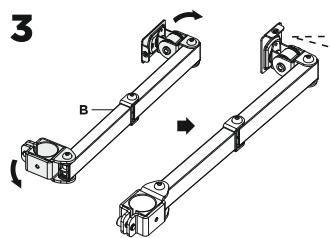
You will need to position the VESA Mounts to an UP position. To do that insert the VESA plate and rotate it to an upright position as shown. When complete, remove the VESA plate and proceed to the next step.
