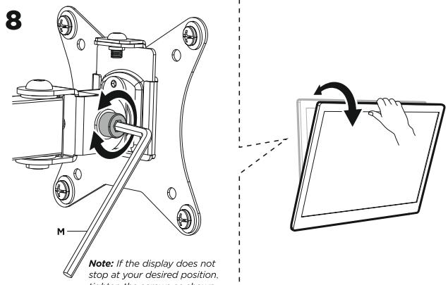
Note: If the display does not stop at your desired position, tighten the screws as shown.
