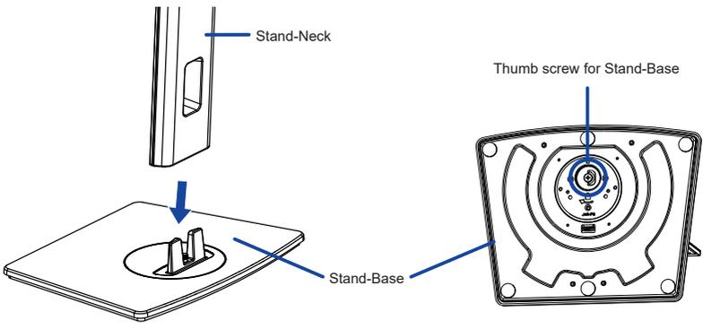
⑤ Hold the monitor and install the assembled stand to the monitor until it clicks to secure.
