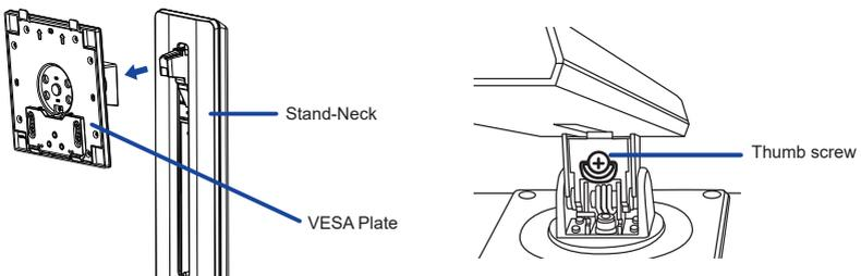
④ Install the Stand-Neck to the Stand-Base and then tighten the 'thumb screw' to secure them.
