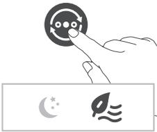
**Natural breeze mode (🍃):** Adjusts fan speeds up and down to mimic the natural movement of air and bring the refreshing feeling of an outdoor breeze into the room.
