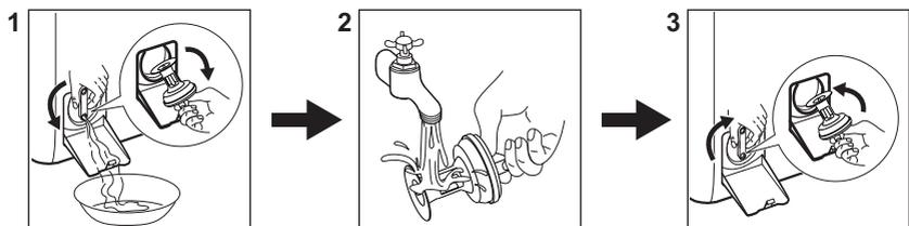
Clean the filter regularly and, especially, if the alarm code **E20** appears on the display.
