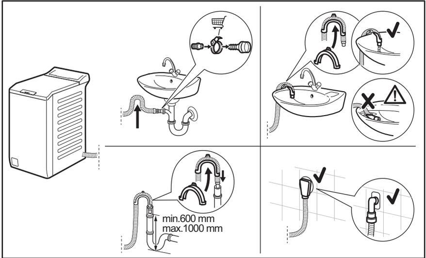
The drain hose should stay at a height of no less than 600 mm and not more than 1000 mm. You can extend the drain hose to maximum 4000 mm. Contact the authorised service centre for the other drain hose and the extension.
