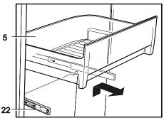
The drawer **5** moves on roller bearings **22**. The drawer can be removed by pulling it out, and lifting it off the rails.
